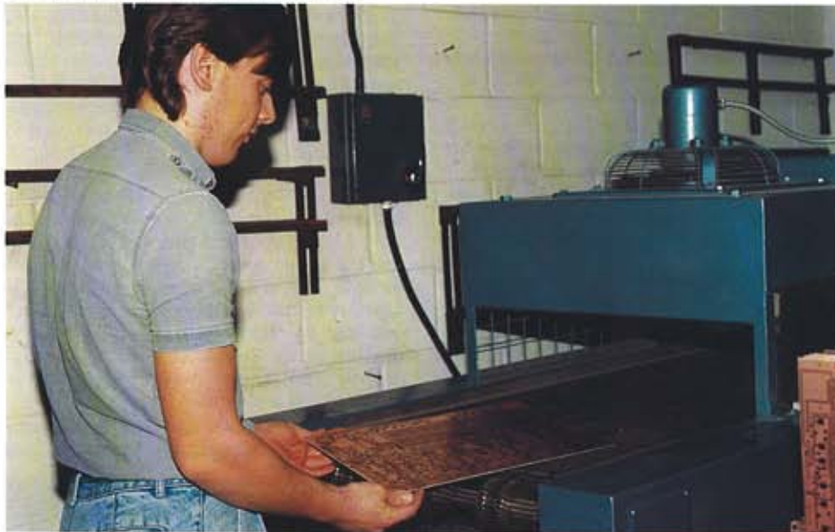
Printed circuit boards flowing through the infra-red dryer. Panels are also printed in this department.
