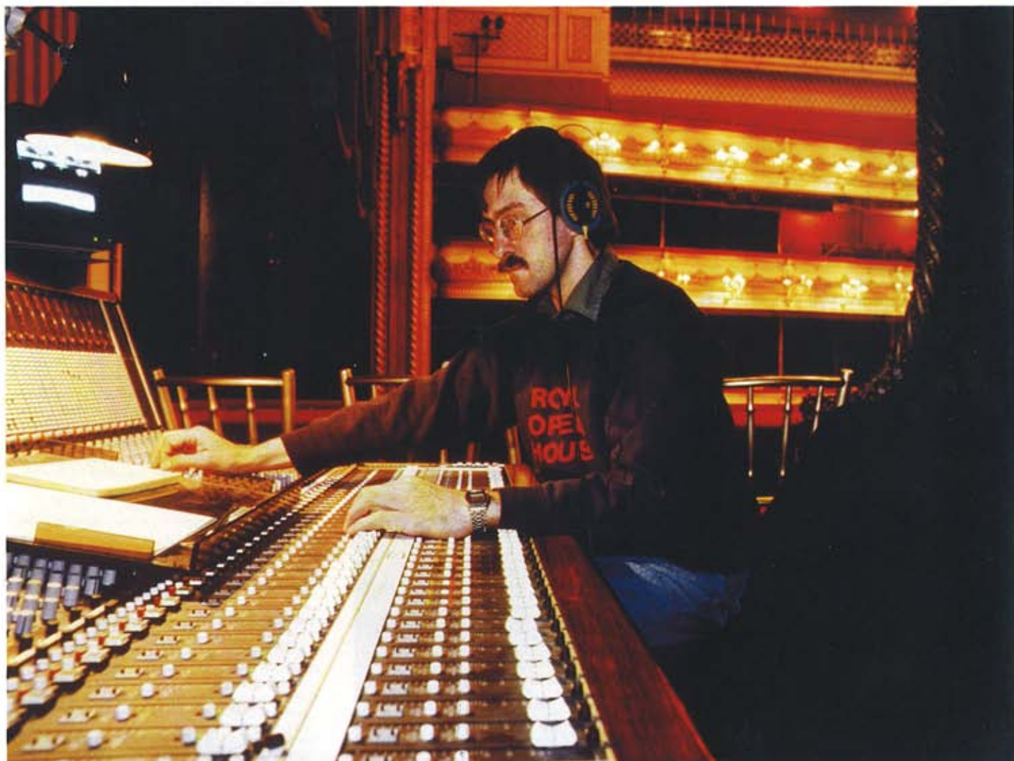
Royal Opera House sound engineer John Charlton pictured at the main mixing desk located in the O.P. side of the auditorium, almost directly opposite the Royal Box and against the proscenium wall at Grand Tier level. The Calrec mixer has forty inputs, forty outputs, and was installed just over a year ago.
