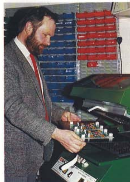
Zero 88's Peter Brooks demonstrates the Vacuclamp. It shrink wraps printed circuit boards in order to keep the components in place so that excess wire can be removed prior to flow soldering.
