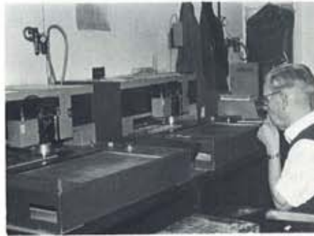
Two computer controlled PCB drilling machines in operation at Pulsar.
